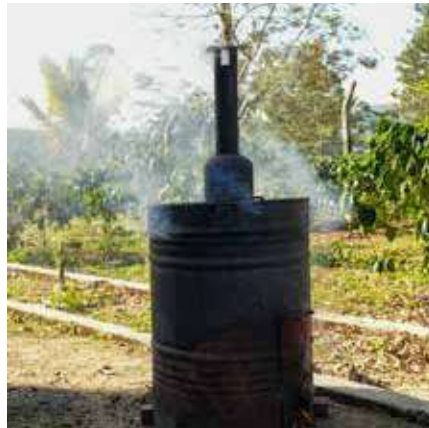
Mini-scale biochar production unit at Mahanilu Estate promoting sustainable soil enhancement
